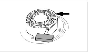
Figure 1. Typical Flywheel Guard Location
